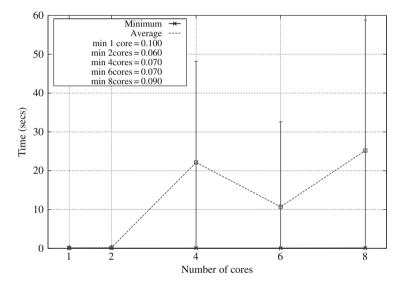
Fig. 21.6 Average execution time of repeated HPL with  $n=1\,\mathrm{k}$  on c1.xlarge instance by number of cores used. The matrices fit within the last-level cache. The input configuration to each execution of HPL is identical. Error bars on average show one standard deviation
