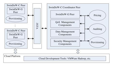
Fig. 13.5 Architecture of SwinDeW-C peers
