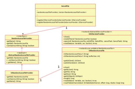
Fig. 26.3 The S3-enabled NetCDF Java interface class diagram
