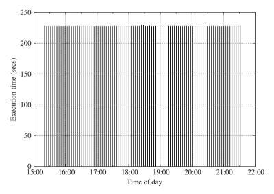
**Fig. 21.2** Execution time of repeated DGEMM using 1 (of 8) core over 6 hours on c1.xlarge instance. Average execution is 227.9 s with a standard deviation of 0.23 s. The input sizes to each DGEMM are identical
