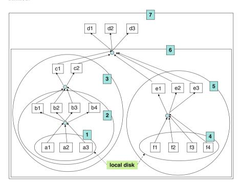
Fig. 9.3 Example machine assignment by workload management
