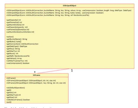
Fig. 26.2 S3StripedObject class diagram
