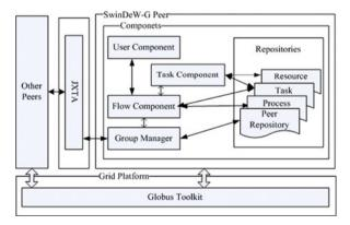
Fig. 13.2 Architecture of a SwinDeW-G Peer
