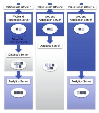
**Fig. 12.2** Vertical load distribution: load can be spread across multiple implementations of the same composite service. This figure illustrates three different implementations of the same service that was shown in Fig. 12.1
