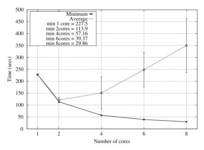
Fig. 21.3 Average execution time of repeated DGEMM with  $n=10\,k$  on c1.xlarge instance by number of cores used. The matrices cannot fit within the last-level cache. The inputs sizes for each DGEMM are identical. Error bars on average show one standard deviation
