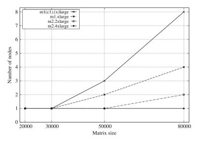
Fig. 21.7 Required number of nodes for different input matrix sizes n. The number of nodes is determined by maximizing usage of RAM on each node. We could not allocate enough m1.large nodes of AMD type to solve a problem of size n=80 k
