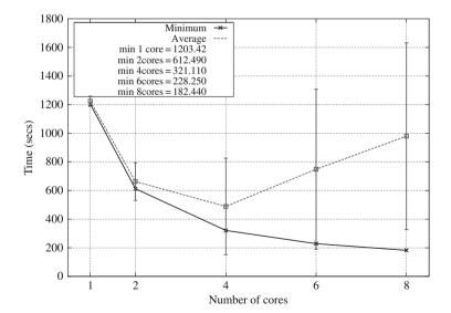
Fig. 21.5 Average execution time of repeated HPL with n=25 k on c1.xlarge instance by number of cores used. The matrices cannot fit within the last-level cache. The input configuration to each execution of HPL is identical. Error bars on average show one standard deviation
