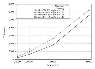
Fig. 21.15 Minimum and average execution time of HPL on m1.xlarge (Opt.) instances by problem size. Error bars on average show one standard deviation
