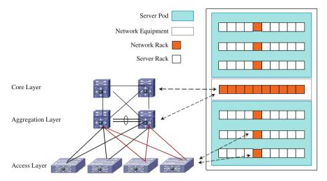
Fig. 4.2 Data center network architecture
