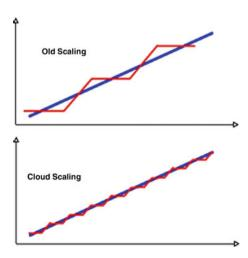
**Fig. 15.4** Cloud computing techniques to reduce overand under-provisioning
