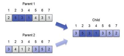
**Fig. 12.7** An example recombination between two parents to produce a child for the first stage assignments. This recombination uses a 2-point crossover recombination of two one-dimensional arrays. Contiguous subsections of both parents are used to create the new child
