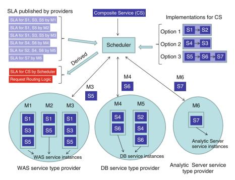
Fig. 12.3 Request routing for SOA-based enterprise computing with multiple implementation options
