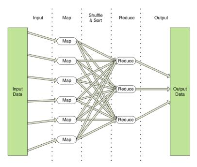
Fig. 5.2 MapReduce processing architecture (O'Malley, 2008)
