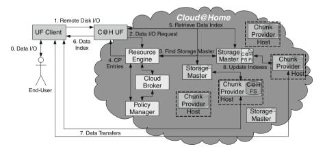
Fig. 25.8 User remote disk I/O request processing
