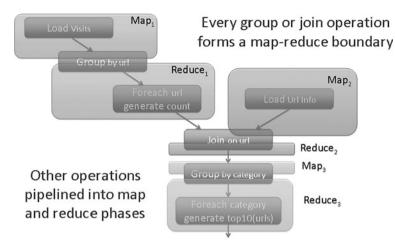
Fig. 5.8 Pig program translation to MapReduce (Olston et al., 2008a)
