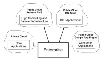
Fig. 1.9 Distributed hybrid cloud architecture (adapted from Lakshmanan (2009))
