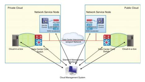
Fig. 4.4 A Functional view of network architecture for hybrid clouds
