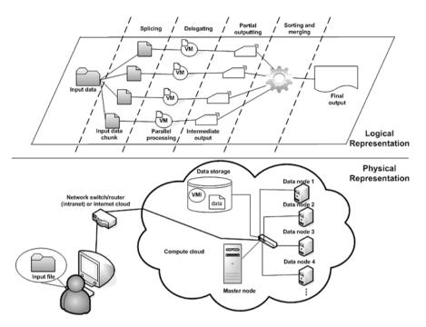
Fig. 23.3 Processing data-intensive scientific task in the cloud
