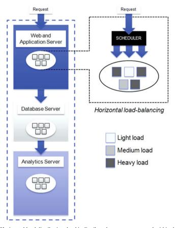
Fig. 12.1 Horizontal load distribution: load is distributed across a server pool within the same tier
