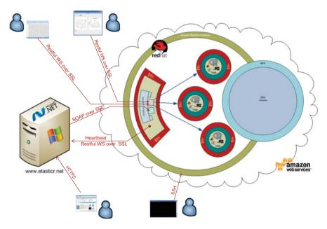
Fig. 19.11 Elastic-R security architecture
