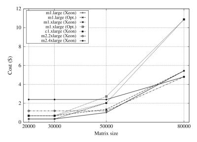
Fig. 21.11 Actual cost to solution for different instance types by problem size. Execution time is rounded to the nearest hour for cost calculation
