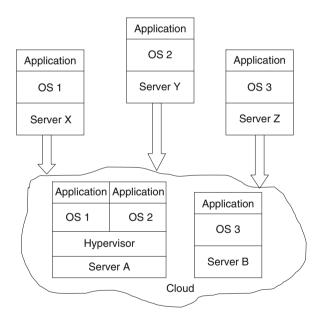
Virtualization technologies include virtual machine techniques such as VMware and Xen, and virtual networks, such as VPN. Virtual machines provide virtualized IT-infrastructures on-demand, while virtual networks support users with a customized network environment to access cloud resources.
