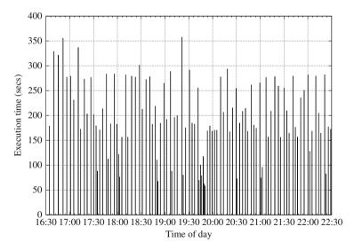
**Fig. 21.1** Execution time of repeated DGEMM using 4 (of 8) cores over 6 hours on c1.xlarge instance. Average execution is 191.8 s with a standard deviation of 68.6 s. The input sizes for each DGEMM are identical. On a stand alone node all executions would be identical
