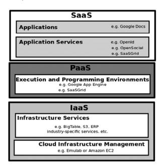
Fig. 15.6 General architecture of the cloud
