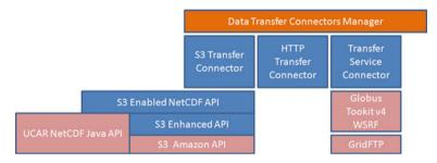
Fig. 26.6 The NetCDF service transfer connector architecture
