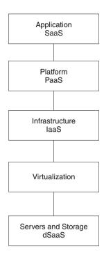
services offered through cloud computing usually include IT services referred as to SaaS (Software-as-a-Service), which is shown on top of the stack. SaaS allows users to run applications remotely from the cloud.
