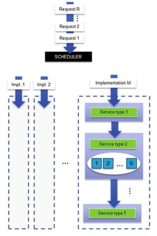
Fig. 12.4 The scheduling and assignment spans two stages. In the first stage, requests are assigned to implementations, and in the second stage, service type instances are assigned to servers
