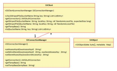
Fig. 26.1 Part of the enhanced S3 Java interface class diagram
