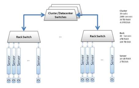
Fig. 15.2 Warehouse-scale system architecture (Barroso & Hölzle, 2009)
