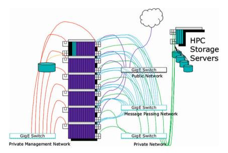
Fig. 11.13 Scalable HPC configuration
