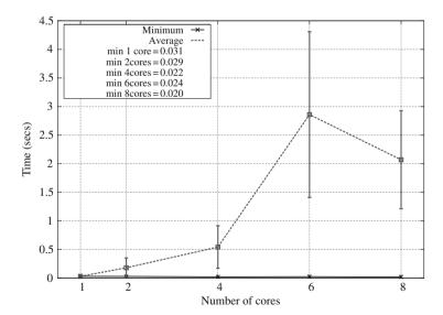
Fig. 21.4 Average execution time of repeated DGEMM with n=500 on c1.xlarge instance by number of cores used. All the matrices fit within the last-level cache at once. The inputs sizes for each DGEMM are identical. Error bars on average show one standard deviation
