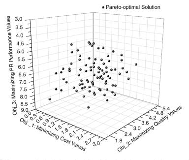
Fig. 17.10 Pareto-optimal solutions of MOGA-IC for simulation example 3 ( $N\!/E=100$  and G=100) obtained by NSGA-II
