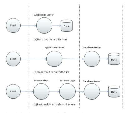
Fig. 15.1 Basic client/server architectures (Orfali et al., 1996)
