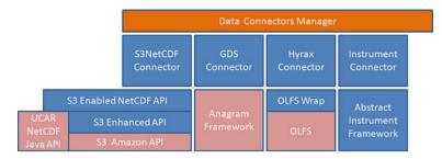
Fig. 26.4 The NetCDF service data connector architecture
