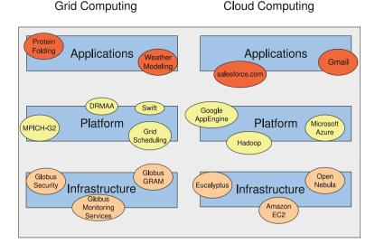
Fig. 8.3 Grid and cloud layers
