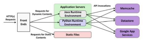
Fig. 14.5 The Architecture of Google App Engine
