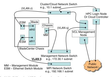
Fig. 11.10 Differentiated HPC node network configuration
