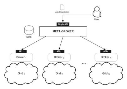
Fig. 8.6 Meta-brokering architecture
