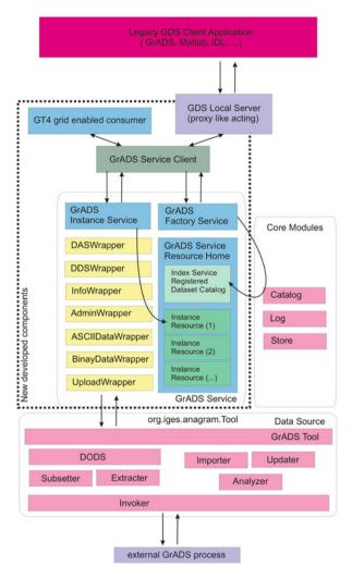
Fig. 20.1 The GrADS Service block diagram
