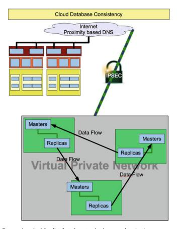
Fig. 24.7 Proposed method for distributed master database synchronization
