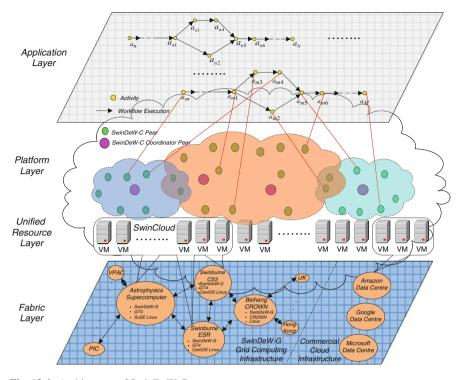
Fig. 13.4 Architecture of SwinDeW-C
